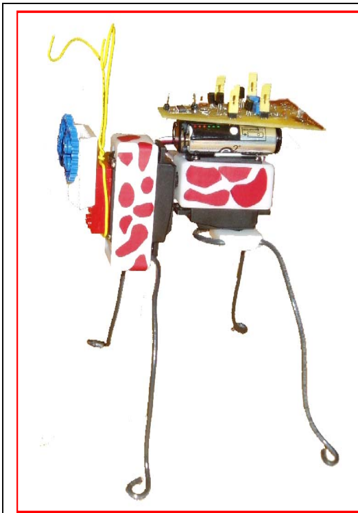
Figure 1. The SlugBug Robot prototype II. The SlugBug is controlled by a neuronal model, implemented with analogues of synapses (real resistors), membranes (real capacitors), and ion channels (real transistors), implementing spiking neurons. The neurons then are linked to behavior by controlling two motors on the robot that make the robot walk.
